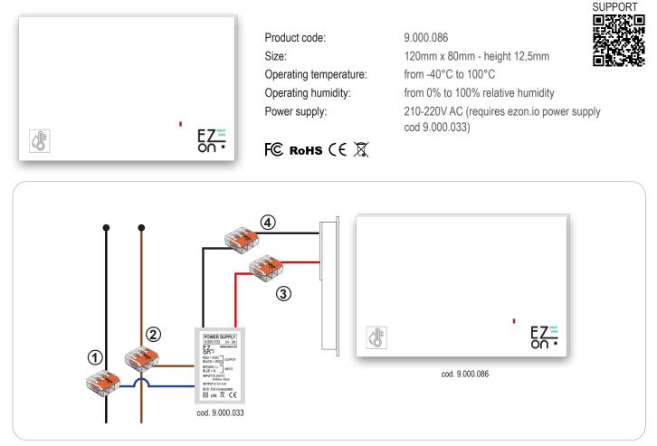
Ezon.io T&H Sensor (for 503) cod. 9.000.086 can determine the temperature and humidity level present in an environment. It is designed to be inserted inside a 503 cassette.
