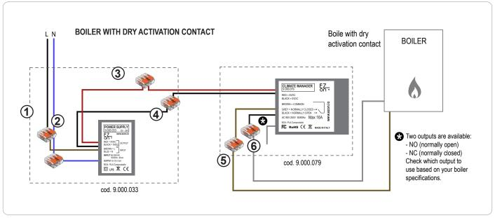
**Ezon.io Climate Manager** cod. 9.000.079 requires a 5VDC power supply to function (we recommend using ezon.io power supply 9.000.033).
