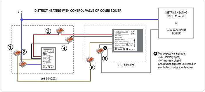
Ezon.io Climate Manager code 9.000.079 requires a 5VDC power supply to function (we recommend using ezon.io power supply 9.000.033).
