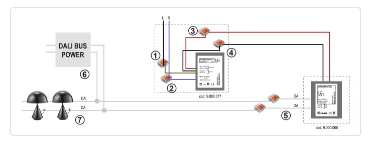
**Ezon.io Dali Bus Power** code 9.000.076 requires a 24VDC power supply to function (we recommend using ezon.io power supply 24V cod. 9.000.077).
