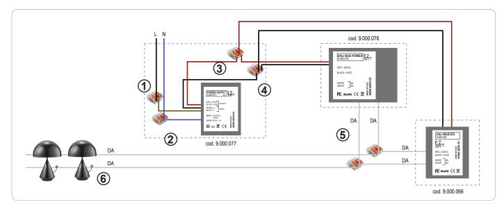
**Ezon.io Dali Master** code 9.000.066 requires a 24vdc power supply to function (the use of ezon.io power supply 24V cod. 9.000.077 is recommended) and a power supply for IEC62386 bus (the use of ezon.io Dali Bus Power 9.000.076 is recommended).
