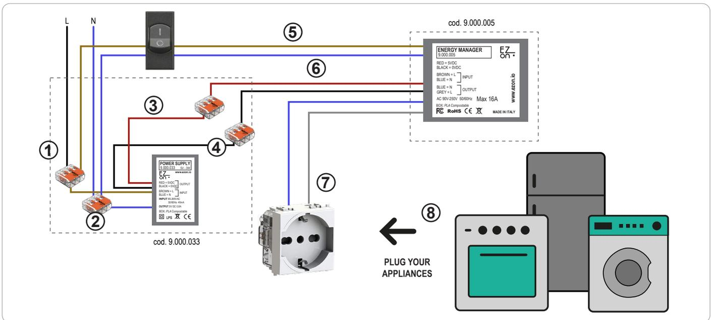
**Ezon.io Energy manager** code 9.000.005 requires a 5vdc power supply to function (the use of the ezone.io power supply 9.000.033 is recommended).
