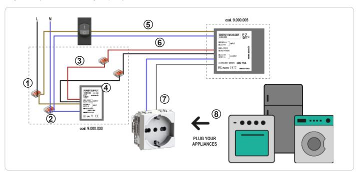
**Ezon.io Energy manager** code 9.000.005 requires a 5vdc power supply to function (the use of the ezon.io power supply 9.000.033 is recommended).
