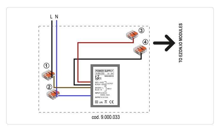
Ezon.io Power Supply code 9.000.033 is a 5vdc power supply, its use is recommended for all ezon.io modules that need to be powered.
