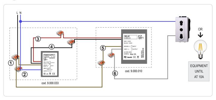
Ezon.io Relay code 9.00 0.010 requires a 5vdc power supply to function (the use of the ezon.io power supply 9.000.033 is recommended).
