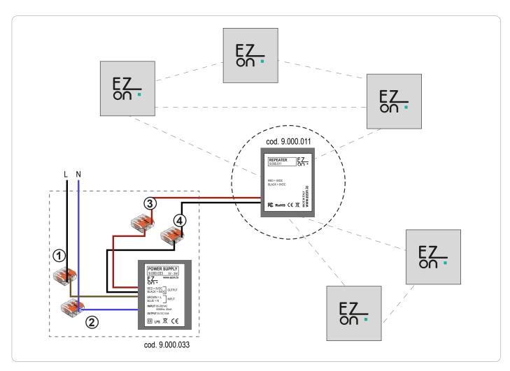
**ezon.io** Repeater it is a signal repeater, in order to function it requires a 5vdc power supply (the use of ezon.io power supply 9.000.033 is recommended).
