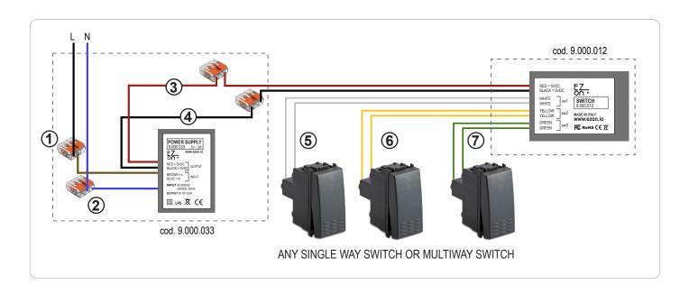
Ezon.io Switch cod. 9.000.012 requires a 5VDC power supply to function (we recommend using ezon.io power supply 9.000.033).
