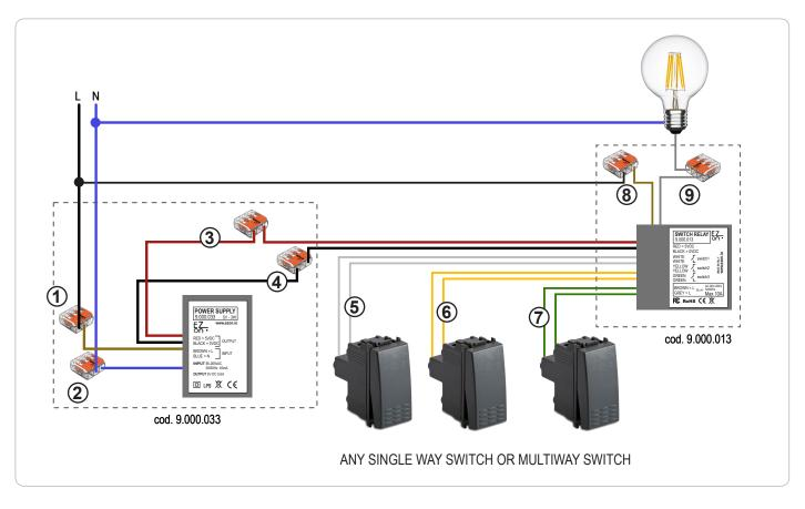
Ezon.io Switch Relay cod. 9.000.013 requires a 5VDC power supply to function (we recommend using ezon.io power supply 9.000.033).
